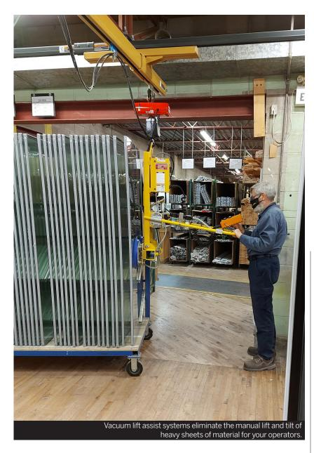
lifting tasks in awkward spaces need to be performed by multiple workers safely, while the use of an electronic lifter or tugger can perform the same task with just one employee without the risk of injury.
